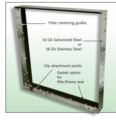
Koch Filter offers the A-8 filter holding frame in several standard sizes. Each can be used individually or in combination to fit just about any size filter bank. Holding frames are available with gaskets, upon request, to seal between filter and frame, minimizing air bypass. Holding frames are available with or without gaskets. Available in 16 gauge galvanized steel and 18 gauge stainless steel.
